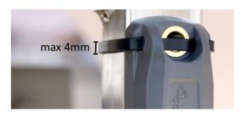
Polarization of Confidex Survivor $^{\text{TM}}$  is according to its longest dimension.
