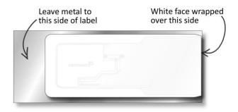
Minimum bending diameter of the Confidex Silverline Classic<sup>™</sup> is 100mm. For optimal performance please bend the label in the orientation shown below.
